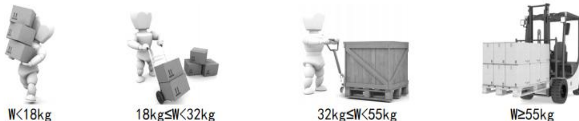
Figure 2-3: Schematic of Lifting Methods for Different Weight Loads
